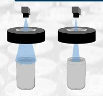
The Vision Inspection Solution for Empty Cans uses a dual circular LED top lighting to illuminate the inspection area for empty can flanges, surfaces and bottoms.
